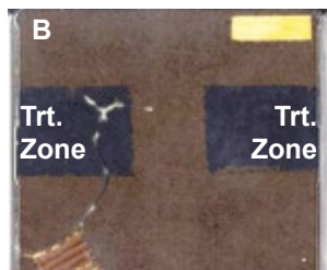
Fig. 2-B. Termidor termiticide/insecticide applications create non-repellent treatment zones around structures, which allow termites to unknowingly forage into these areas, thus acquiring a lethal dose.
